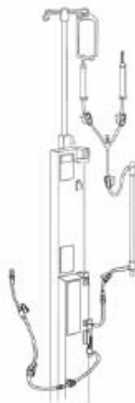
Figure 1: Do not install heat exchanger onto the Fluid Warmer, but install the rest of the set. D-100 is shown. Other sets will vary in spike numbers and clamp locations.
